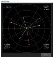
Display two simultaneous vector views of three-phase power systems and correlate them to acquired voltage, current and other waveforms and calculated per-cycle Waveforms.
