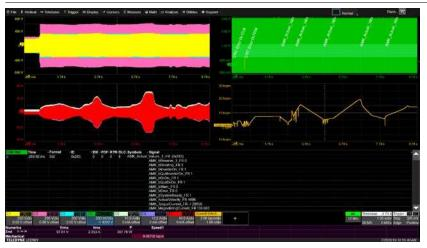
Speed data is extracted from digital CAN-encoded serial data and plotted as an analog speed per-cycle Waveform, as if the signal was directly probed.
