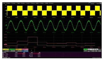
This simplified example shows THD for voltage and current (bottom magenta and orange Waveforms) plotted over time with one THD value per power cycle.
