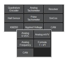
14 different methods to calculate speed, angle and torque - most supported only by the Motor Drive Analyzer.
