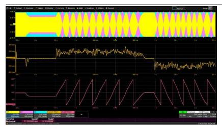
Speed and angle are calculated from the analog sine, cosine and excitation frequency signals of a resolver, with user-defined angle tracking observer applied.
