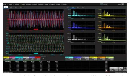
Capture and calculate harmonics during very short or long acquisitions and show results as Spectral Waveform displays, total THD values or per-cycle THD Waveforms.
