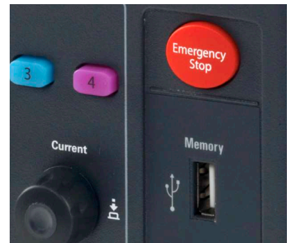
Figure 12. The emergency stop button shuts down all outputs immediately.
