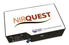
The NIRQuest (Near Infrared) Fiber Optic Spectrometer combines the high-performance InGaAs array detector with the high-sensitivity NIRQuest optical bench. The NIRQuest Spectrometer and the 16-bit A/D converter share a single housing, forming a small-footprint plug-and-play system.
