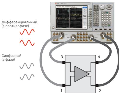
$$\begin{bmatrix} S_{DD 11} & S_{DD 12} & S_{DC 11} & S_{DC 12} \\ S_{DD 21} & S_{DD 22} & S_{DC 21} & S_{DC 22} \\ S_{CD 11} & S_{CD 12} & S_{CC 11} & S_{CC 12} \\ S_{CD 21} & S_{CD 22} & S_{CC 21} & S_{CC 22} \end{bmatrix}$$
