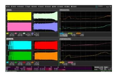
This 480V drive has 10 second acquisitions for the AC Input and Drive Output (on the left) and on the right are shown power, efficiency and power factor Waveforms over time.
