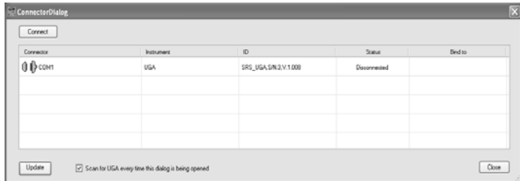
Fig. 2-14. Screenshot of UGA control software after selecting 'Connect' in the Main menu. The available Serial connector is shown.
