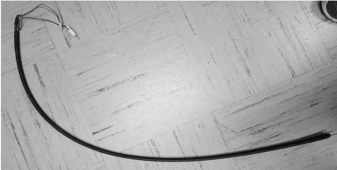
Fig 1-9. Capillary with heater. The connector for heater power and TC is also shown.
