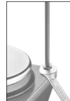
Note: When using bath attachments with a diameter over 180 mm, please use support rod in conjunction with an extension. (See "Accessories")
