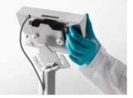
Place your terminal on a stand which is quickly mounted at the back of your balance. The display is easier to read and good posture is maintained.
