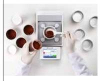
Under standard conditions, 1 mg readability balances with SmartPan can be used without a draft shield. In a fume cupboard, the draft shield doors can be left open during weighing-in. Process steps are reduced, and weighing is faster and more ergonomic.
