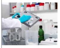
The innovative SmartPan weighing pan and drip tray underneath dismantle easily. Any spilled substances remain in the tray for safe disposal and easy cleaning.
