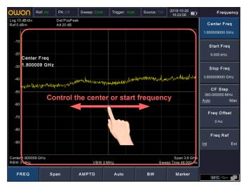
●Set the Span (Span→[Span]): In the display area, pinch and spread horizontally to change the span.
