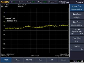
Figure 3-10 Full Span
