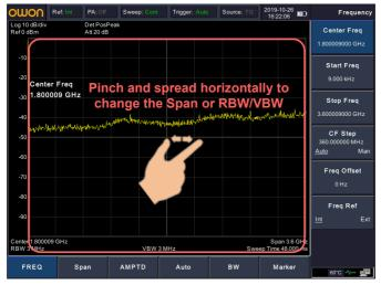
●Set the Scale/Div (AMPTD → [Scale/Div]): In the display area, pinch and spread vertically to change the Scale/Div.
