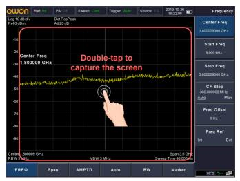
•Move the active marker to the desired frequency (Marker  $\rightarrow$  [Marker  $\triangleright$ ]  $\rightarrow$  turn the knob): When a marker is active, single-tap in the display area (at any level) to quickly move the marker to the desired frequency.
