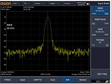
Figure 3-11 Set frequency span
