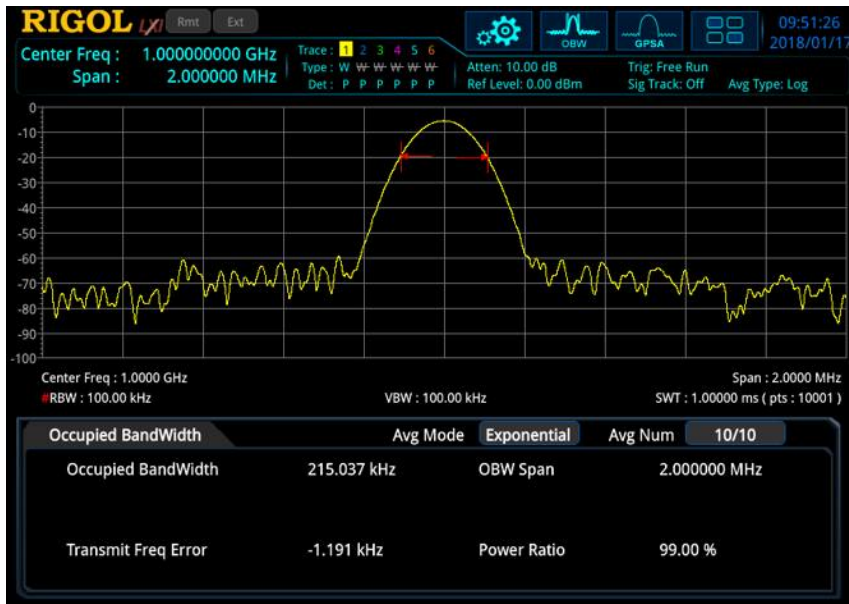
Figure 2-8 OBW Measurement Interface
