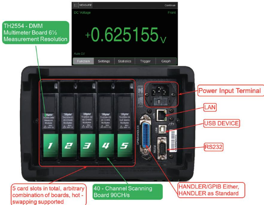
The TH2554 is equipped with common interfaces such as RS232, USB HOST, USB DEVICE, and HANDLER, and supports the standard SCPI command set, making it suitable for automated integration.
