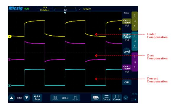
Figure 2-14 Probe Compensation
