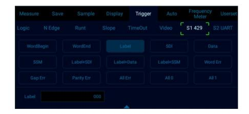
Figure 12-27 ARINC429 Trigger Mode Configuration Menu
