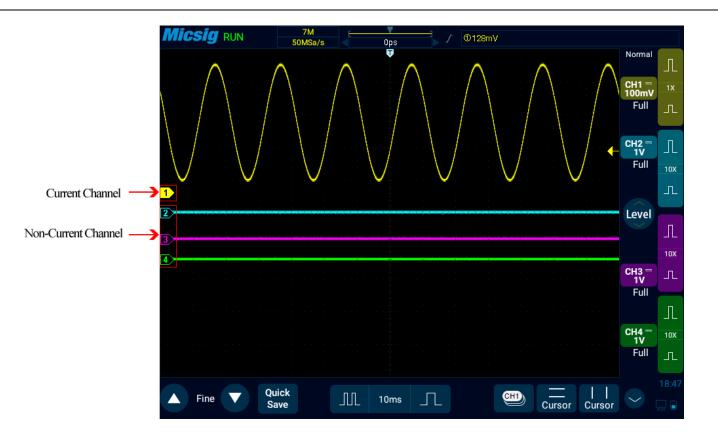
Figure 5-2 Current Channel and Non-Current Channel
