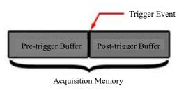
Figure 6-6 Conceptual Demonstration of Acquisition Memory
