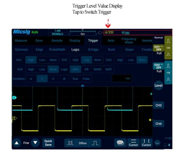
Figure 6-21 Trigger Level Adjustment
