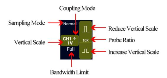
Figure 5-3 Channel Display Interface
