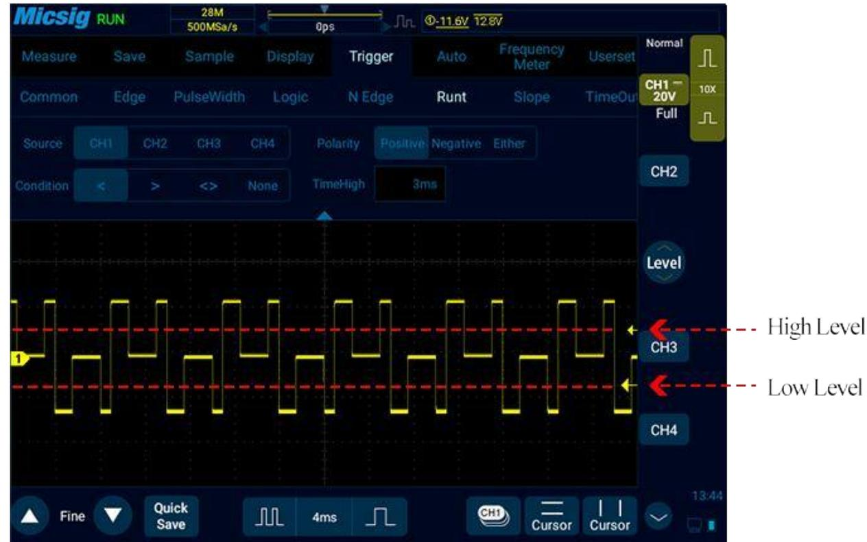
Figure 6-24 Runt Trigger Setting Menu
