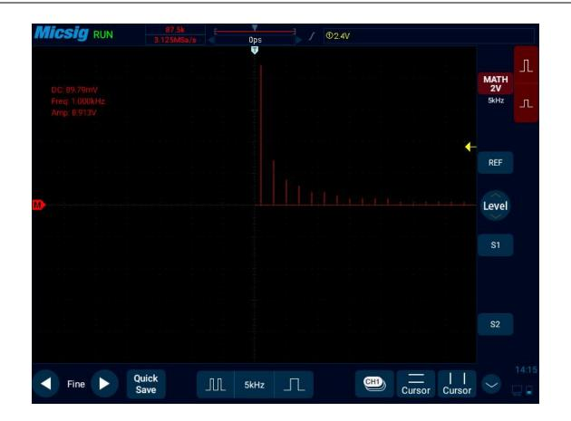
Figure 9-4 Spectrum Amplitude as V-Hz
