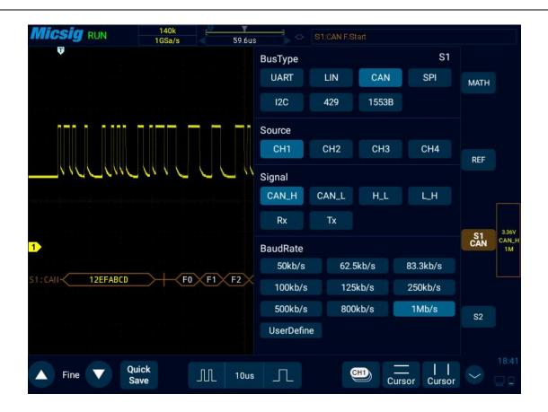
Figure 12-14 CAN Bus Configuration Menu
