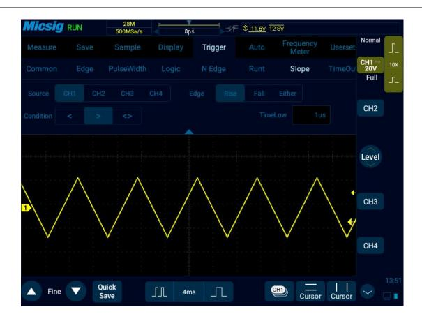
Figure 6-26 Slope Trigger Setting Menu
