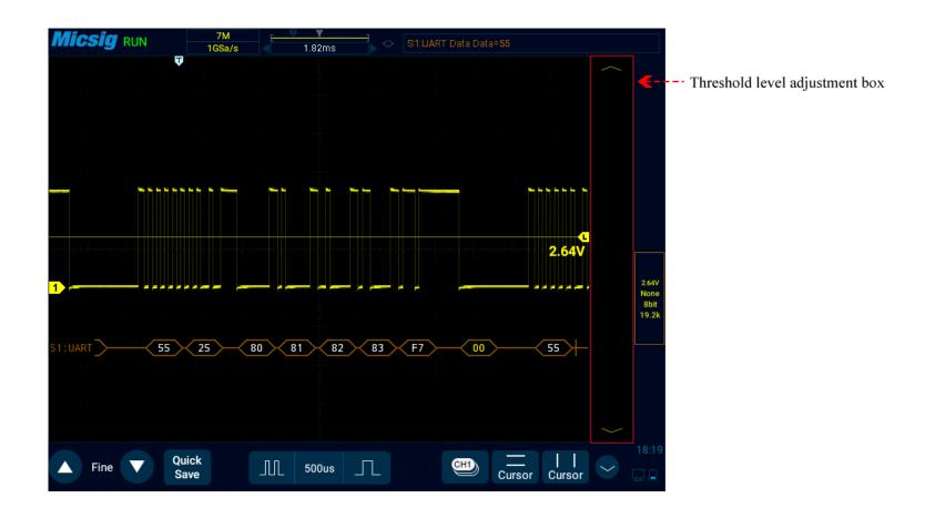
Figure 12-7 UART Decode Level Adjustment
