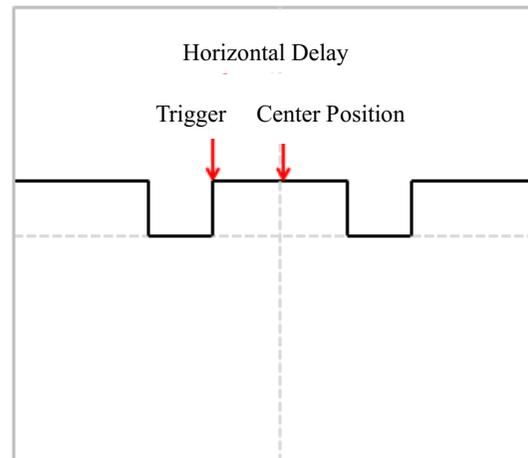
Figure 6-7 Horizontal Delay
