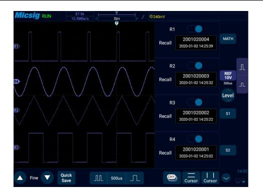
Figure 9-6 Restore Reference Waveform
