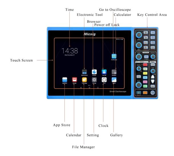
Figure 2-4 Front Panel of Tablet Oscilloscope
