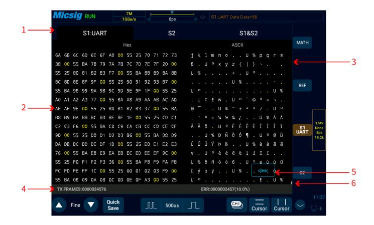
(5) When "?" appears, the time base needs to be adjusted to view decode results.
