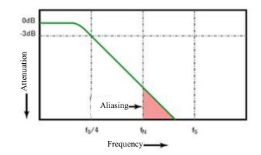
Figure 11-3 Sampling Rate and Oscilloscope Bandwidth
