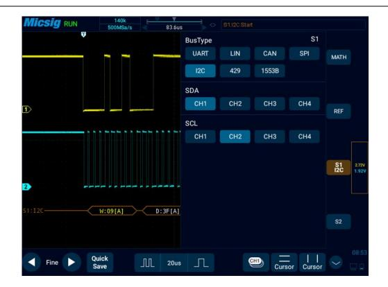
Figure 12-22 I2C Bus Configuration Menu
