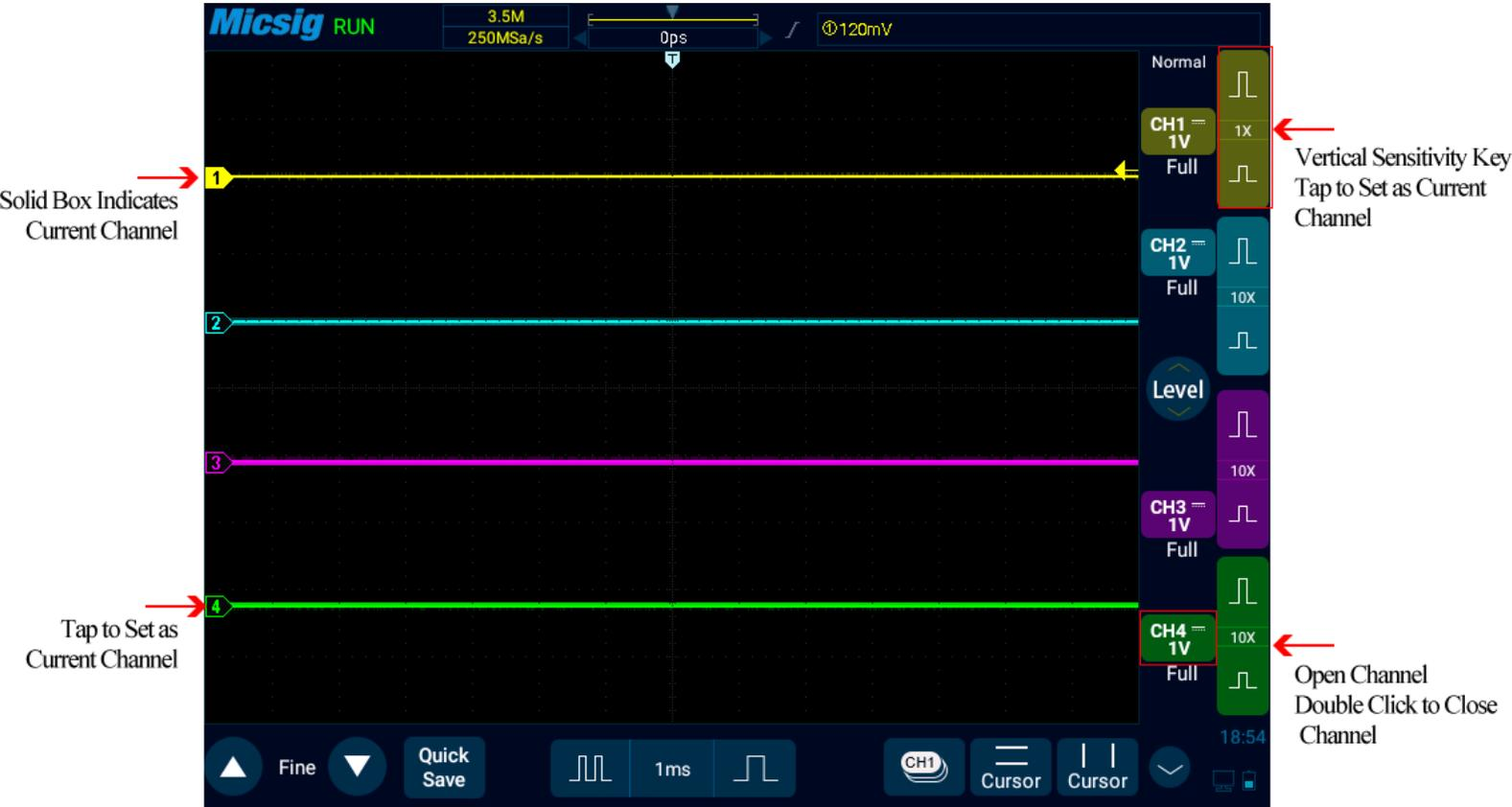
Figure 5-4 Channel Open, Close and Switching
