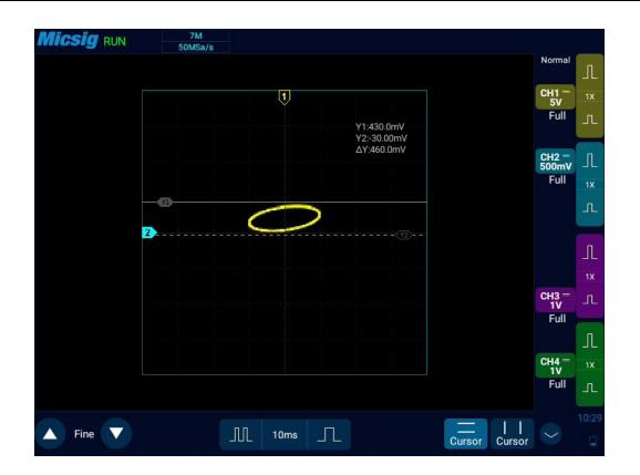
Figure 4-10 Phase Difference Measurement and Using the Cursor
