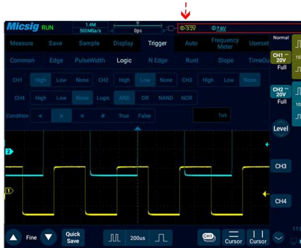
Figure 6-21 Trigger Level Adjustment
