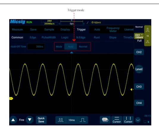
Figure 6-5 Oscilloscope Trigger Mode Setting
