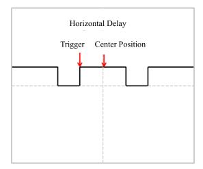
Figure 6-7 Horizontal Delay
