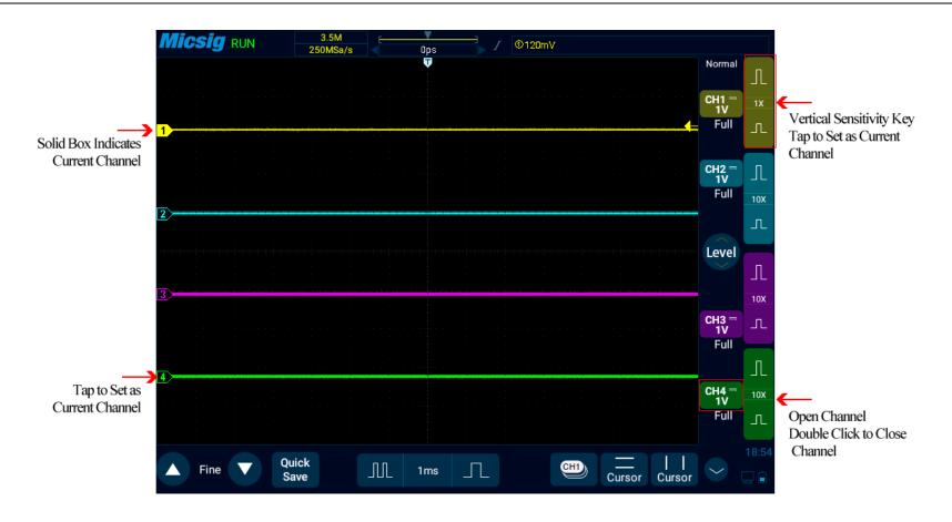
Figure 5-4 Channel Open, Close and Switching
