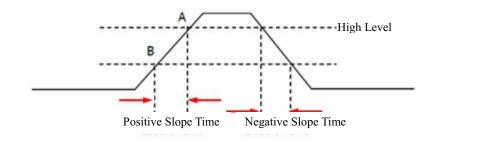
Figure 6-25 Positive/Negative Slope Time
