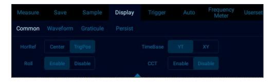
Figure 4-7 Roll Mode On/Off
