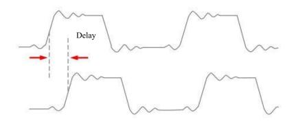
Figure 7-5 Delay Measurement Schematics
