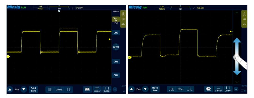
Figure 6-3 Abnormal Signal in Periodic Signals
