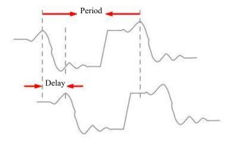
Figure 7-6 Phase Measurement Schematics
