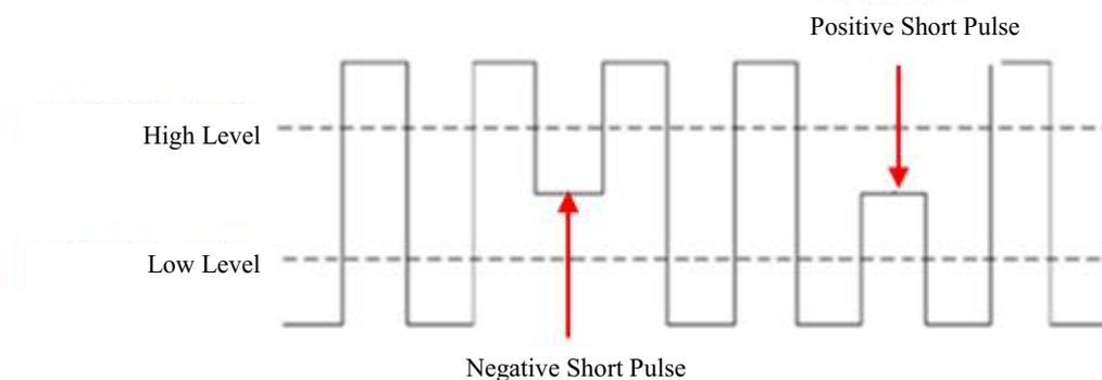
Figure 6-23 Runt Trigger
