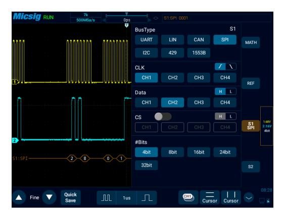
Figure 12-18 SPI Bus Configuration Menu
