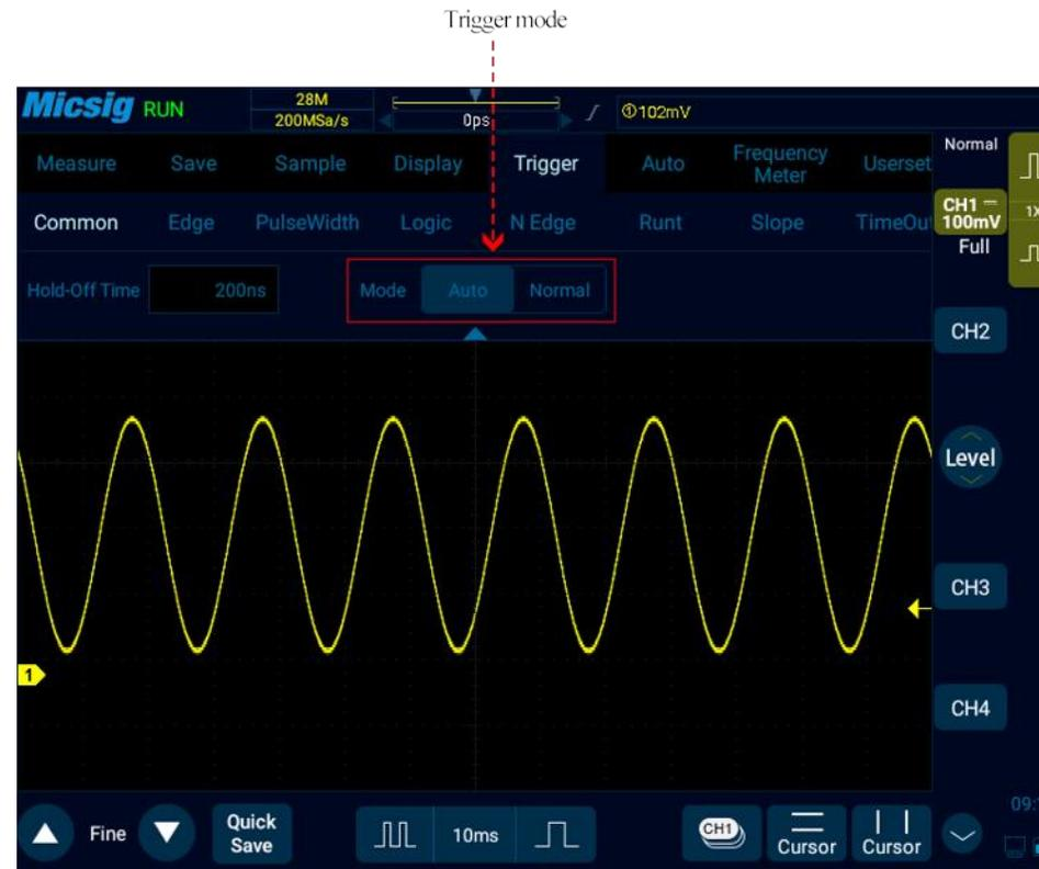
Figure 6-5 Oscilloscope Trigger Mode Setting
