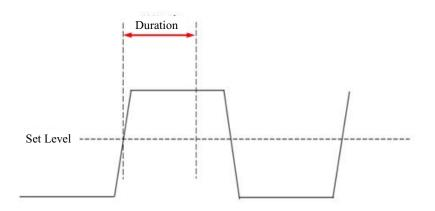
Figure 6-27 Timeout Trigger Schematics
