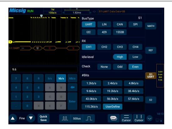
Figure 12-5 Baud Rate Default Setting
