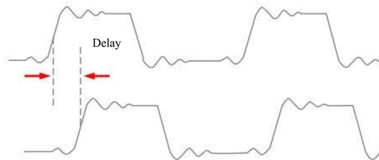
Figure 7-5 Delay Measurement Schematics
