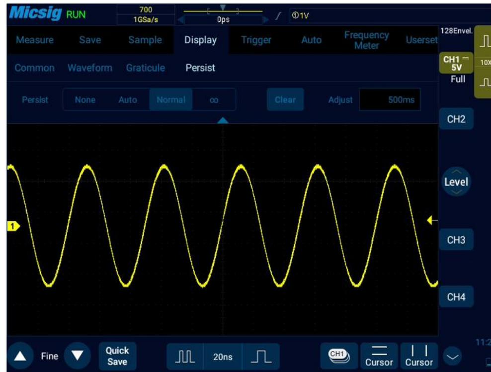
Figure 10-4 20MHz Sine Wave Variable Persistence 500ms
