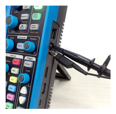
Figure 2-13 Probe Connection
