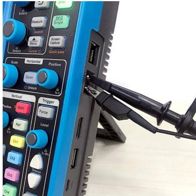
Figure 2-13 Probe Connection
