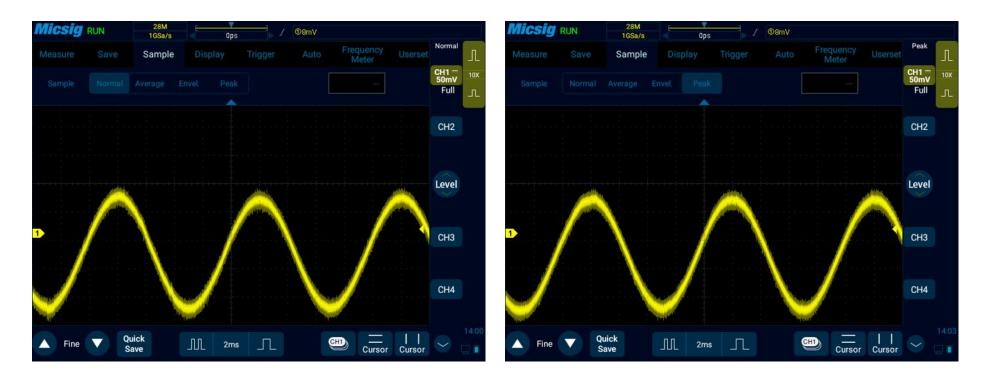
Figure 11-5 Sine Wave with Burr
