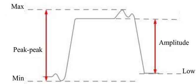
Figure 7-7 Voltage Measurement
