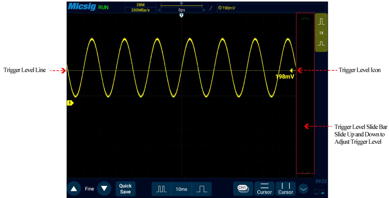
Figure 6-8 Trigger Level
