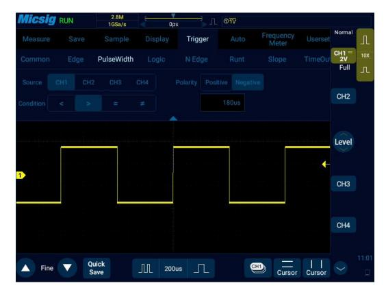
Figure 6-14 Negative Polarity Pulse Level Flip
