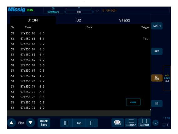
Figure 12-21 SPI Text Interface
