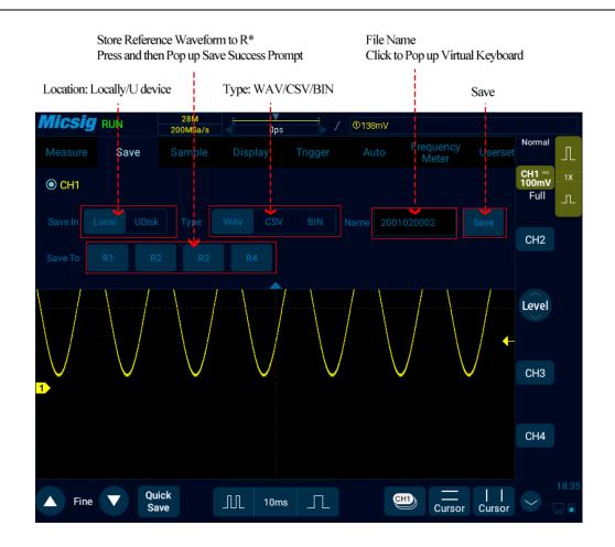
Figure 8-4 Save CH1 Reference Waveform Interface
