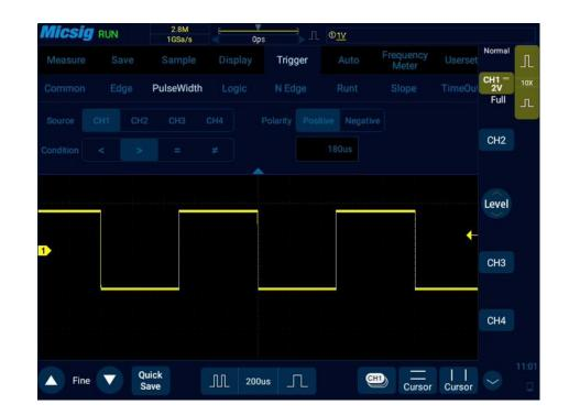
Figure 6-13 Pulse Width Trigger Setting Menu
