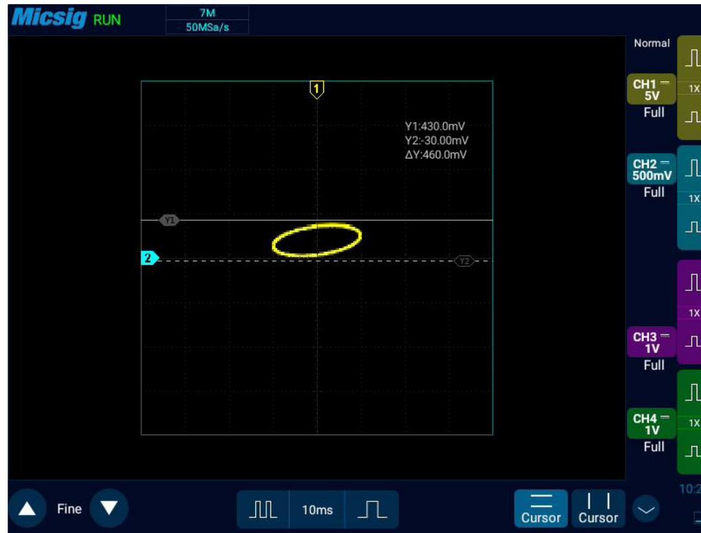
Figure 4-10 Phase Difference Measurement and Using the Cursor
