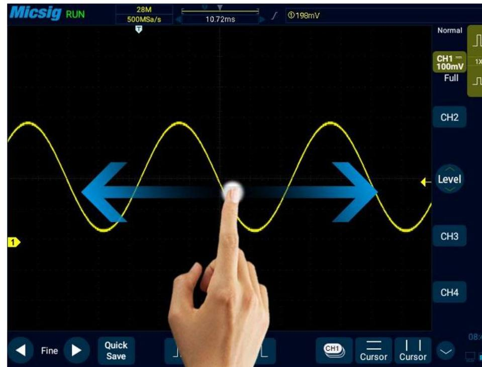
Figure 4-2 Move the Waveform Horizontally on the Screen
