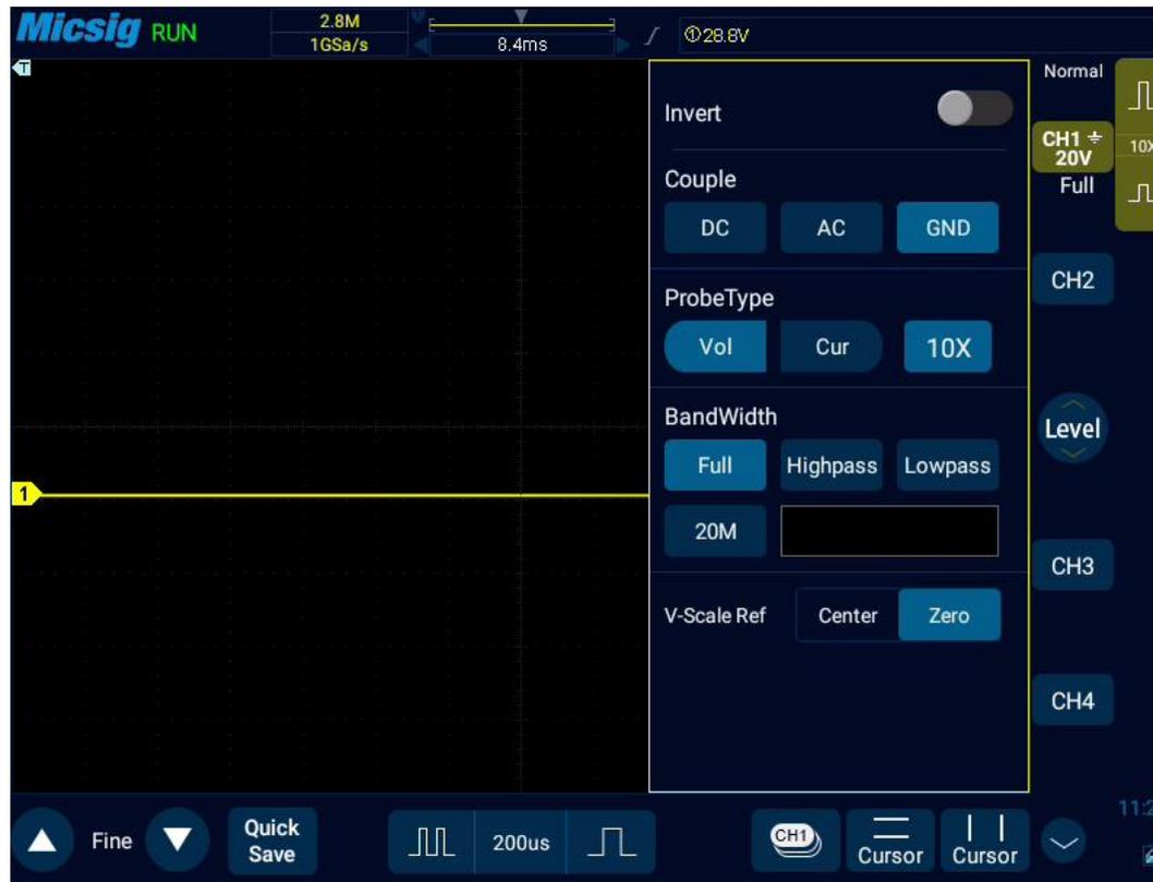
Figure 5-9 GND Coupling
