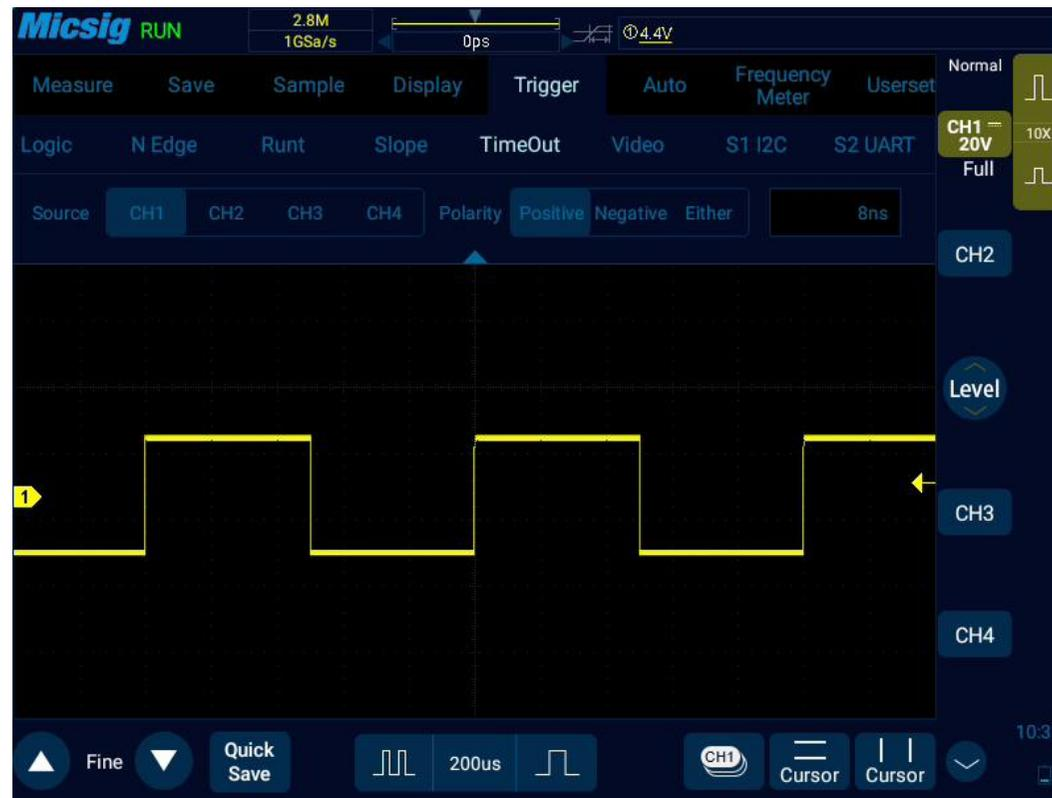
Figure 6-28 Time-out Trigger
