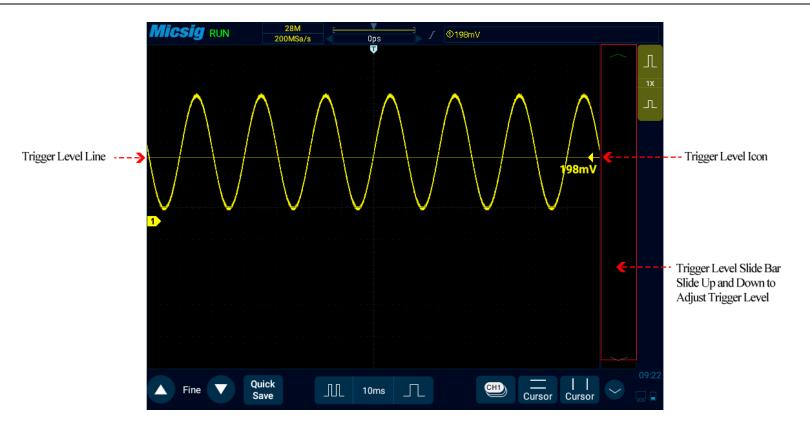
Figure 6-8 Trigger Level
