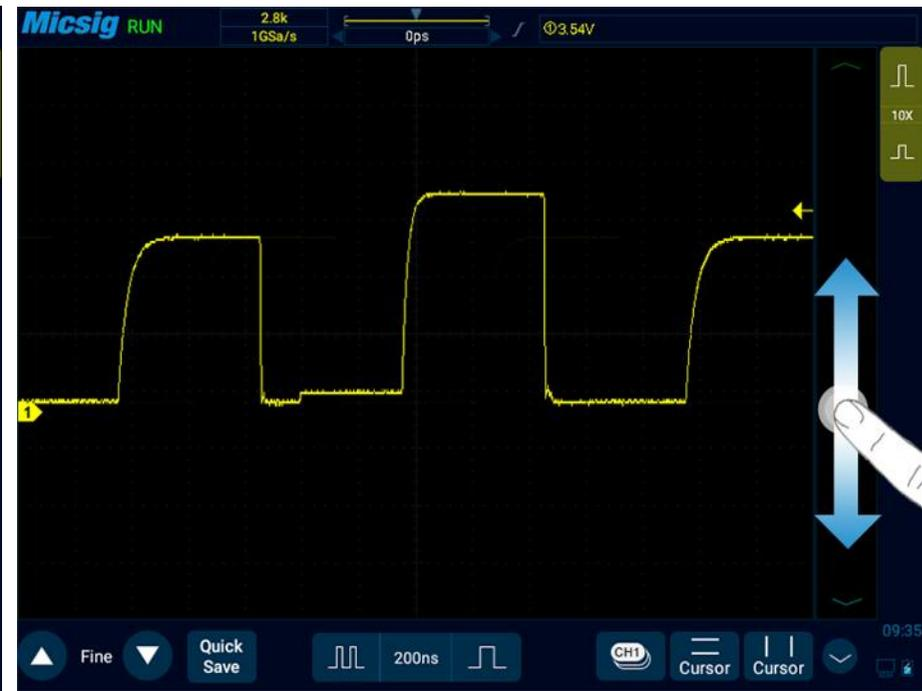
Figure 6-4 Abnormal Signal Captured by Setting Trigger Level
