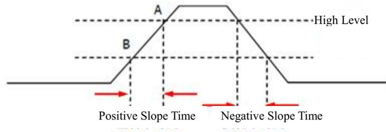
Figure 6-25 Positive/Negative Slope Time
