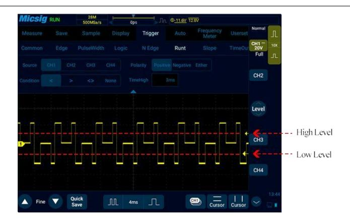
Figure 6-24 Runt Trigger Setting Menu
