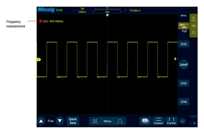
Figure 7-9 Frequency Meter Measurement
