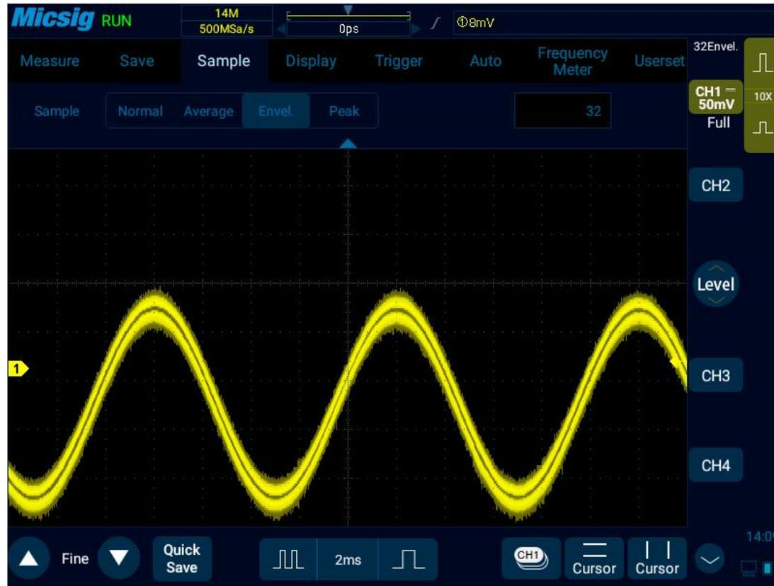
Figure 11-8 AM Signal in Envelope Sampling Mode (32)
