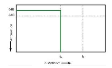
Figure 11-2 Theoretical Brick-Wall Frequency Response
