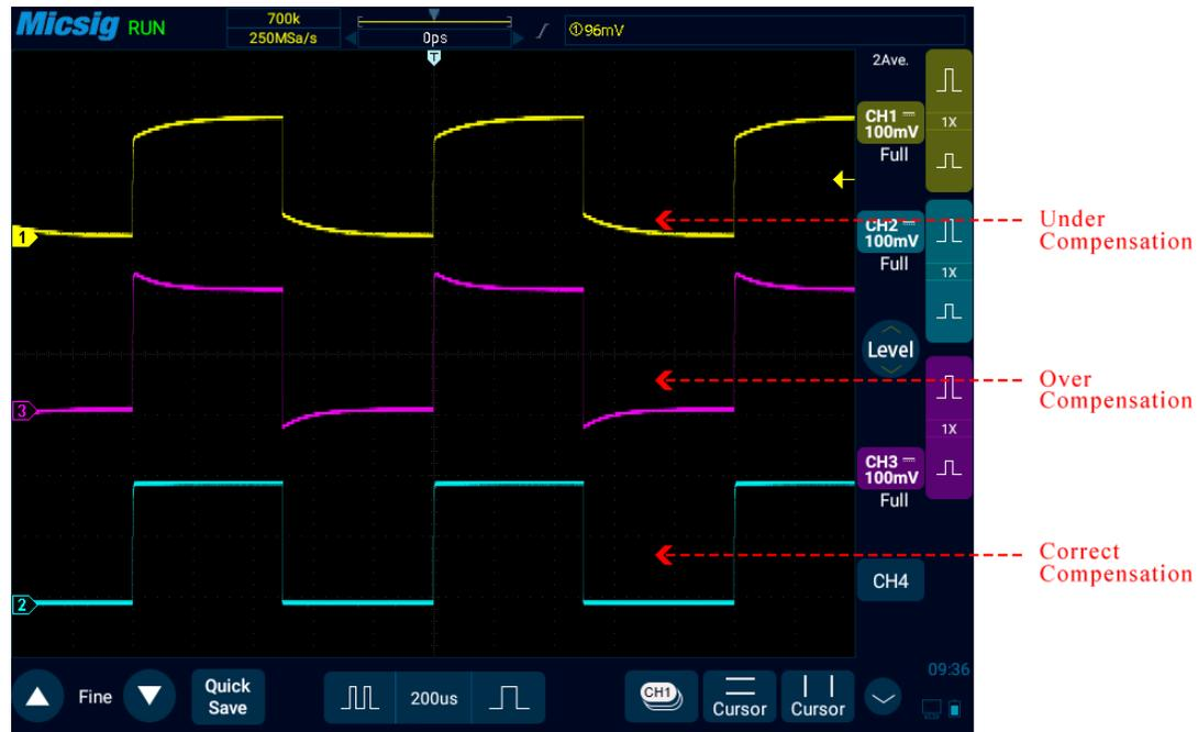
Figure 2-14 Probe Compensation
