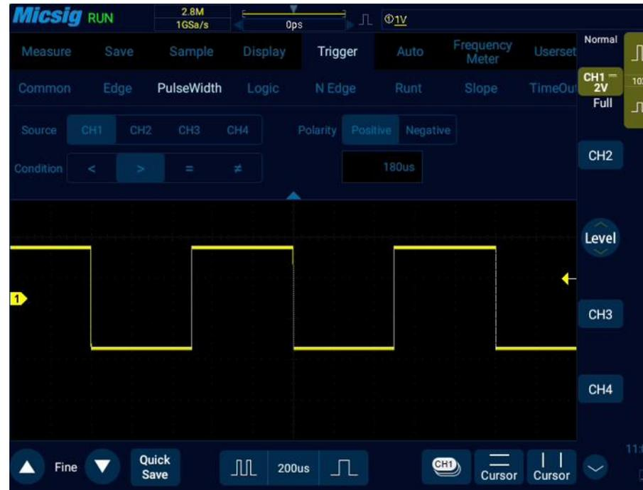
Figure 6-13 Pulse Width Trigger Setting Menu
