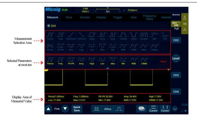
Figure 7-1 Automatic Measurement Menu
