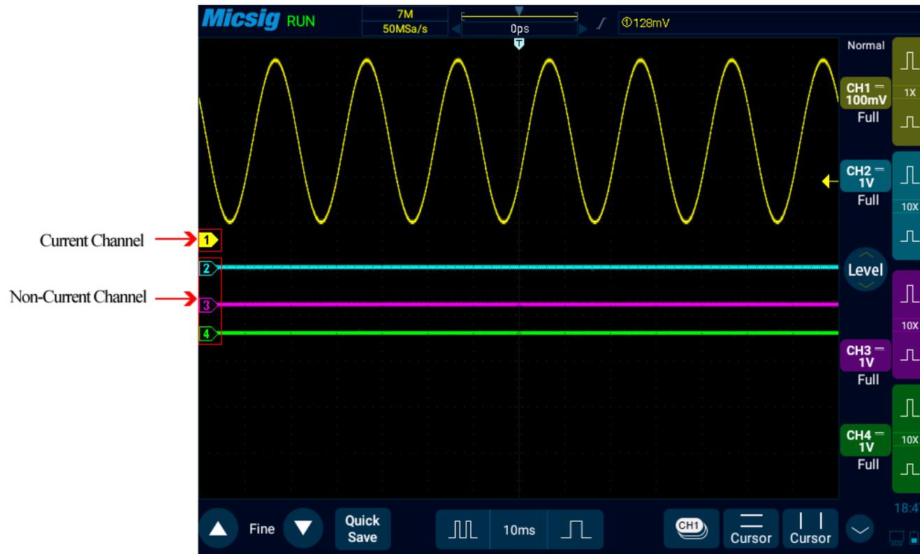
Figure 5-2 Current Channel and Non-Current Channel
