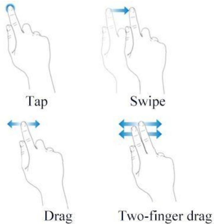
Figure 2-6 Basic Operations of Smart Oscilloscope
