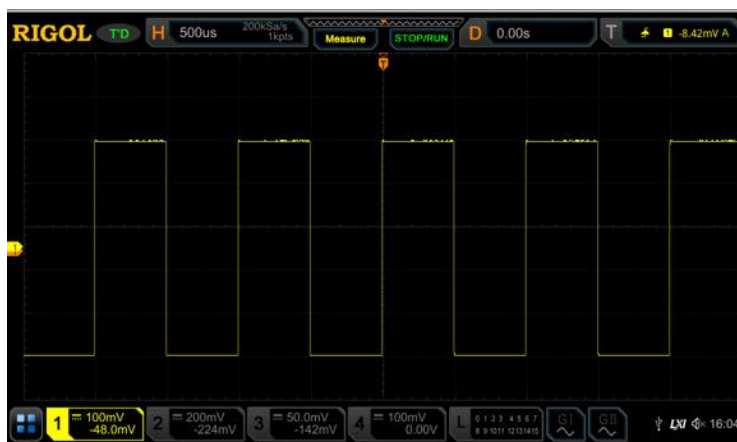
Figure 4-3 Waveforms after 128 Times of Averaging
