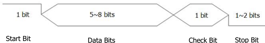
Figure 5-13 Schematic Diagram of RS232 Protocol
