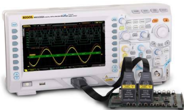
Figure 1-6 To Connect the Logic Probe
