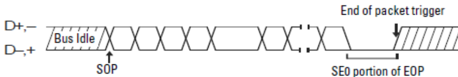
Figure 5-9 USB Data Transmission Protocol
