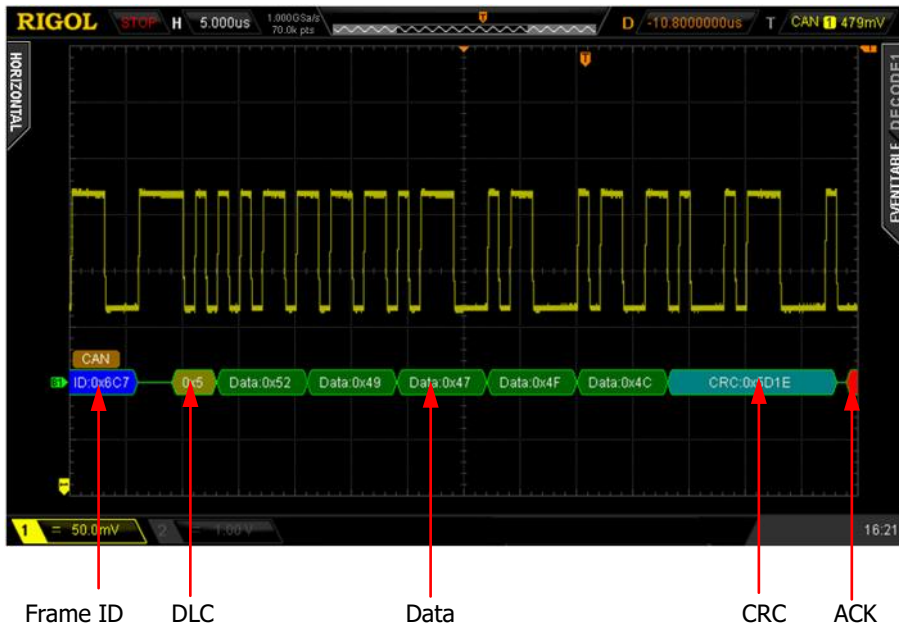
Figure 7-15 Decoded CAN Data Interpretation
