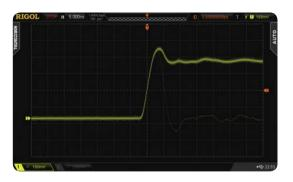
UltraVision: multi-level intensity grading display (256-level)
