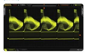
Abundant advanced triggering functions (e.g. Runt Trigger, Setup/Hold Trigger, and Nth Edge Trigger)
