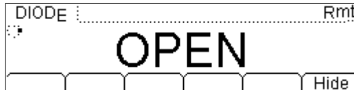
Figure 2-28 Testing interface of Diode
