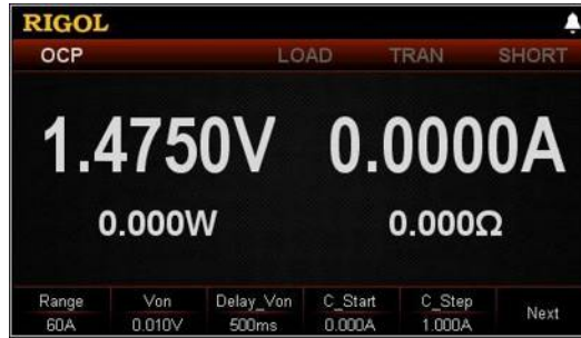
Figure 2-30 Main Interface of OCP Test Function
