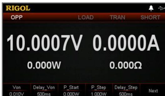
Figure 2-34 Main Interface of OPP Test Function
