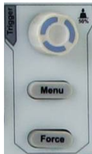
Figure 3-13 Trigger Control Zone
