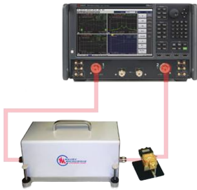
Block diagram of a four-port N5245B PNA-X with test set option 423, and low-noise receiver option 029. A Maury Microwave's LXI tuner is used as an impedance tuner to provide a wide-range of source impedances.
