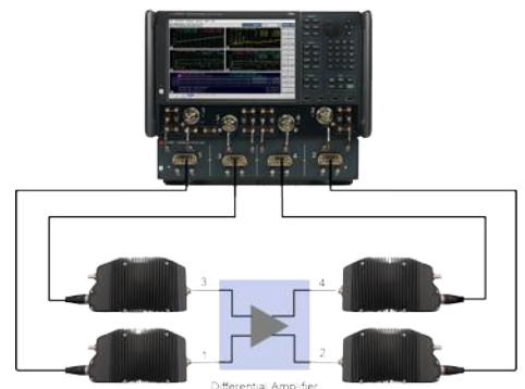
True-differential measurement of a balanced trans-impedance amplifier using a four-port PNA, the N5292A controller, and N5293A frequency extenders.
