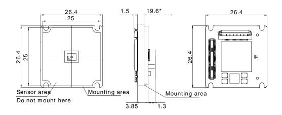
$^{\ast}\mbox{Mechanical}$  distance from the mounting area to the C-Mount front flange
