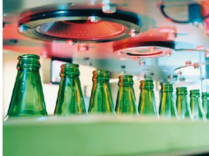
View of a row of an empty bottle inspection system, which uses pixelfly cameras for the improved resolution inspection (IRIS), courtesy of Kronen AG, Neutraubling, Germany
