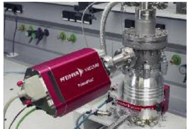
PrismaPlus on a residual gas analysis system
