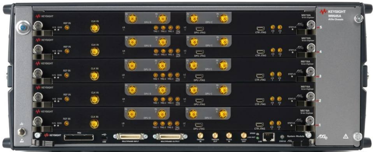
Figure 3. Five M9710A digitizers installed in the M9505A 5-slot chassis, forming a 20-ch 10-bit acquisition system.
