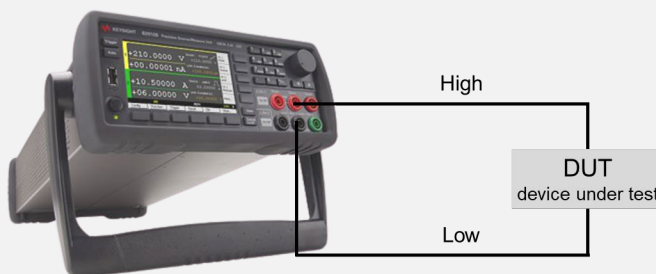
Same measurement using an SMU
