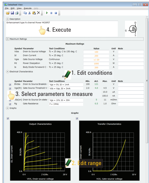
The intuitive data sheet characterization mode of Easy Test Navigator provides complete device characteristics in a few simple steps
