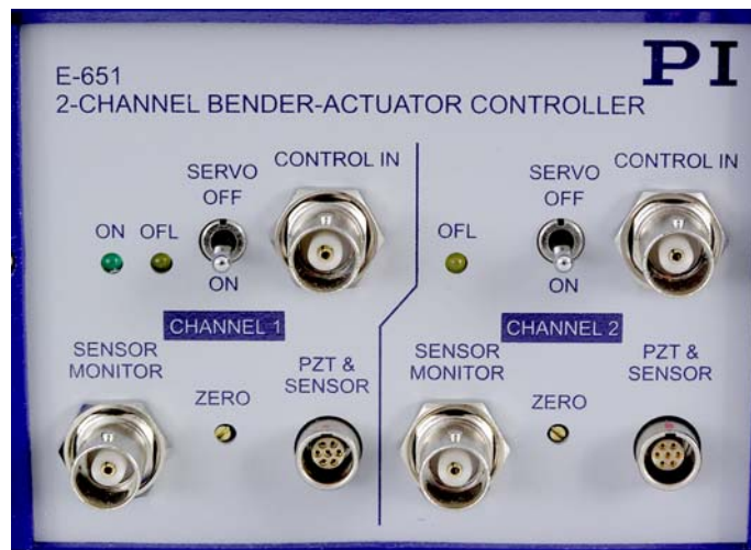
Fig. 3: E-651 front panel; elements for channel 2 are not present on single-channel models
