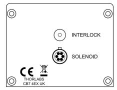
Fig. 3.2 Rear Panel Connections
