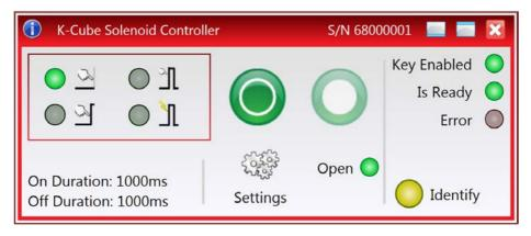
Fig. 6.1 Solenoid Controller K-Cube Software GUI
