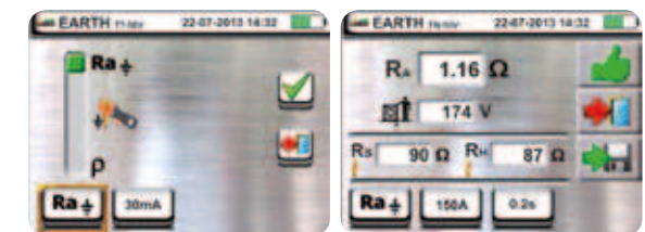
Earth resistance measurement by Volt-ampere method
