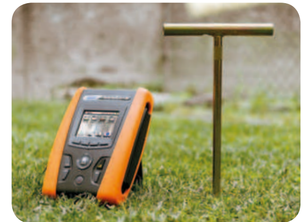
Earth resistance measurement by Volt-ampere method
