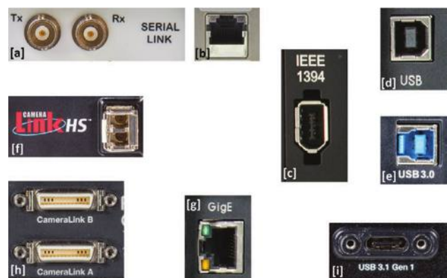
Figure 1: Photos of a variety of image data interface connectors: [a] proprietary highspeed serial data interface based on coaxial cables, [b] proprietary highspeed serial data interface based on LAN cables, [c] IEEE 1394 a “Firewire” interface, [d] USB 2.0 interface (device side), [e] USB 3.0 interface (device side), [f] Camera Link HS interface, [g] Gigabit Ethernet interface, [h] Camera Link Full interface and [i] USB 3.1 Gen 1 interface.
